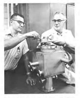
IT'S METRIC — first all metric job out of the machine shop was completed by Jim Myers (left) and Joe Shelby (both 3644-2). The unit, a vacuum chamber with a turret mechanism to hold samples (on top)/(held by Joe), "proves that even a guy with 36 years of working with inches can adjust to millimetres," says Joe. Adds Jim, "We're getting more metric tools and converting more machines all the time." The chamber was constructed for Dal Jensen (2413) with drawings by Johnny Baca (9611).
